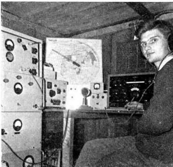
The overall winner was S. J. Pilkington (G3NNT) of Ormskirk, Lancashire. The transmitter, on the left of the picture, has an 813 in the p.a. The aerial is a cubical quad for 14, 21 and 28 Mc/s.
